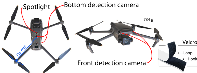
Fig. 18. Illustration of the quadrotor platform (DJI MAVIC3). The front and bottom cameras are used for detection. The gimbal camera was not selected for detection since its dedicated designed for photography and with high link delay. The drone and the surface are secured with velcro after perching.
