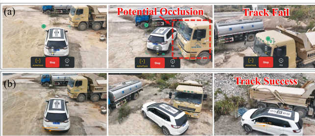
Fig. 19. Comparison with the origin DJI tracking under scenario 2. (a) Active tracking function of DJI MAVIC loses the target car at the turning. (b) Our tracking scheme enhances visibility actively, tracking successfully.
