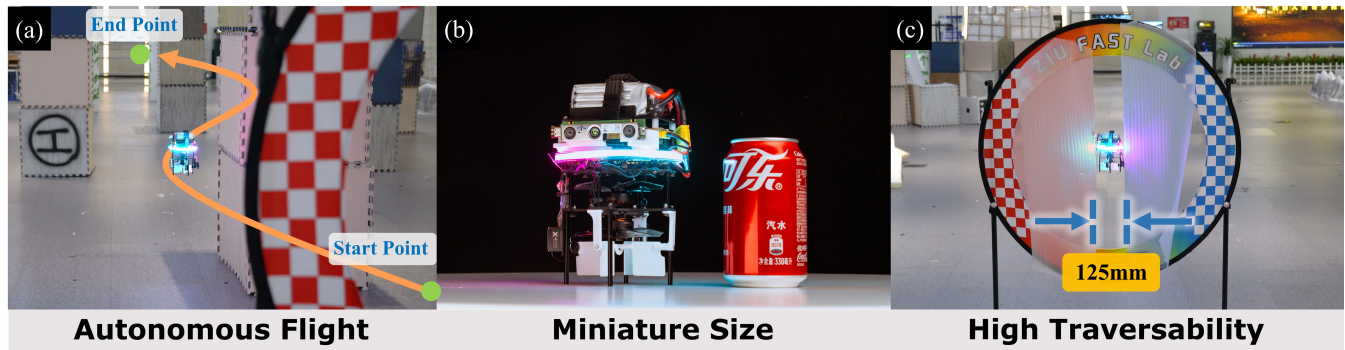
Fig. 1: The proposed coaxial helicopter (a) autonomously navigates through an unknown cluttered environment, (b) possesses a miniature size slightly larger than a can of soda, (c) deftly crosses through a narrow gap of 125mm wide.
