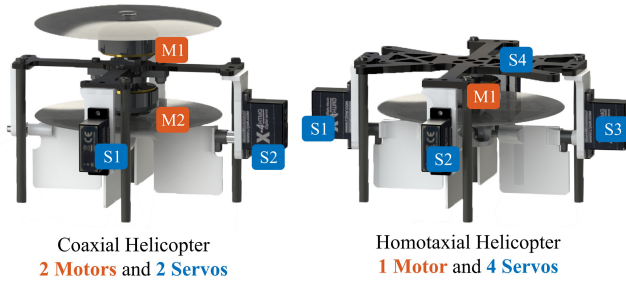
Fig. 5: The comparison between a coaxial helicopter and a homotaxial helicopter.
